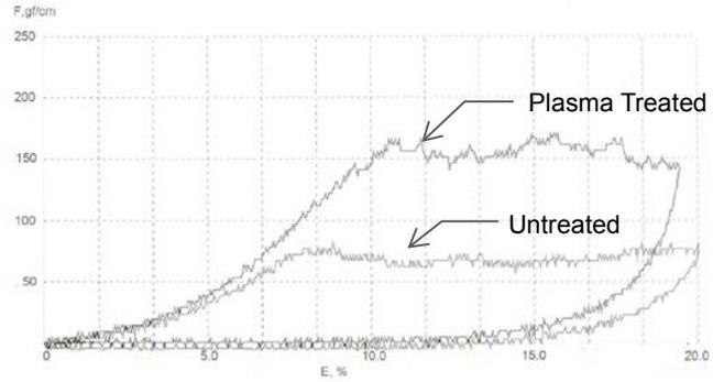
Fig. 3-2 Example of Measurement of Peeling Strength Using KES-FB1 Tensile Tester
