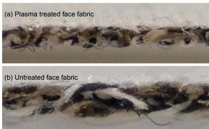
Fig.5 Cross-Section of Bi-Fabrics (a) Plasma Treated Face Fabric, (b) Untreated
