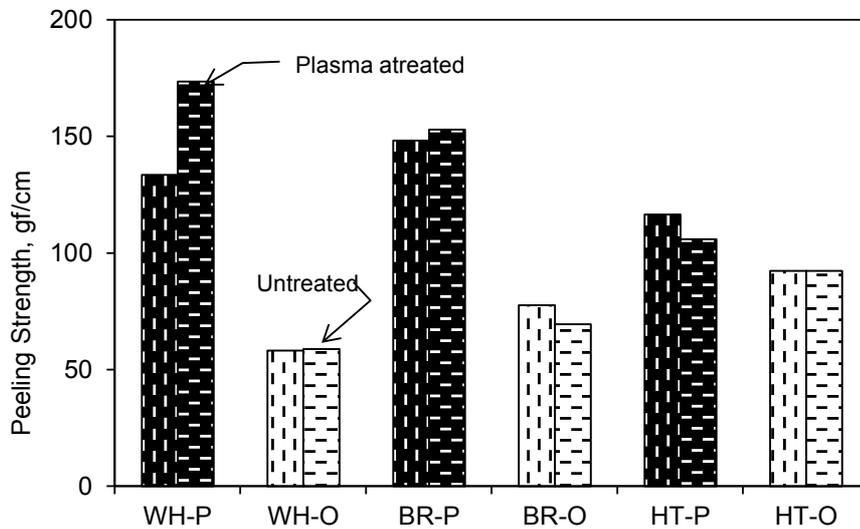
Fig. 4 Peeling Strength for Three Fabric Samples (Warp and Weft Directions)
